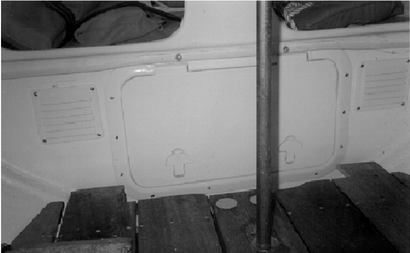
Photo 6.2 “Sunny II” Battery Box and Tabernacle Support
